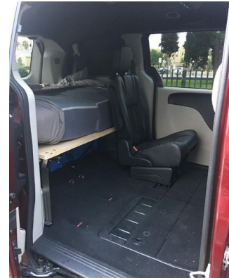
5. Set one or both middle seats up - to prevent the front panel from lodging forward upon a sudden brake. Always return one or both of the middle seats to upright position before driving the van with a folded bed.
