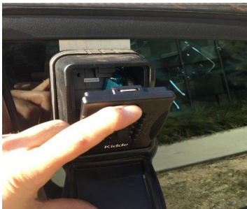
5. While pressing down the lever, pull the cover towards you to open. Once you release the lever, you will need to re-enter in the code.
