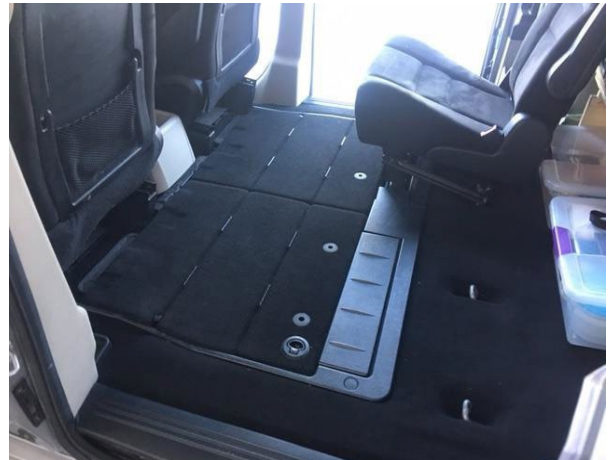
8. Close floor cavity cover
