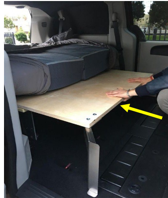
4. Push the front panel between the mattresses and the middle panel. Felt pads on the bottom of the panel facilitate a smooth glide you may have to wiggle it or lift the mattresses slightly to assist.
