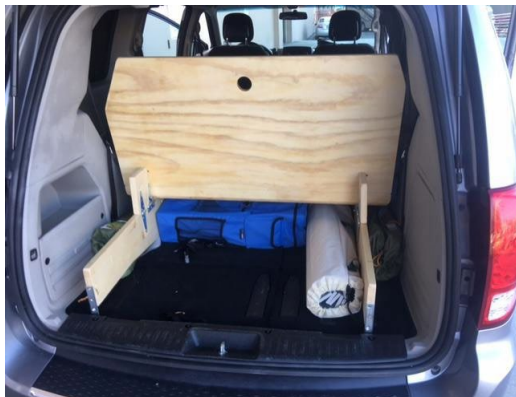
4. Rest rear section on support flaps. In some beds latches are available to secure the flaps in position
