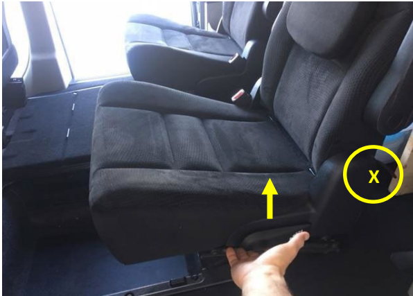
5. Pull the handle upward all the way. The seat will spring forward and fold.
